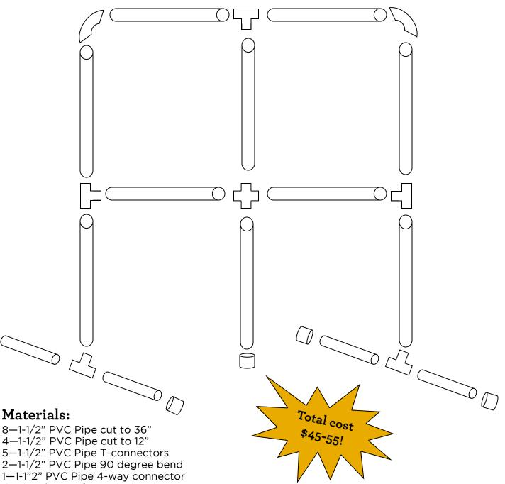
1—1-1"2" PVC Pipe 4-way connector Optional: 5—1-1/2" PVC Pipe Caps 2—Full-size flat sheets of desired color (we recommend black for at least one)
